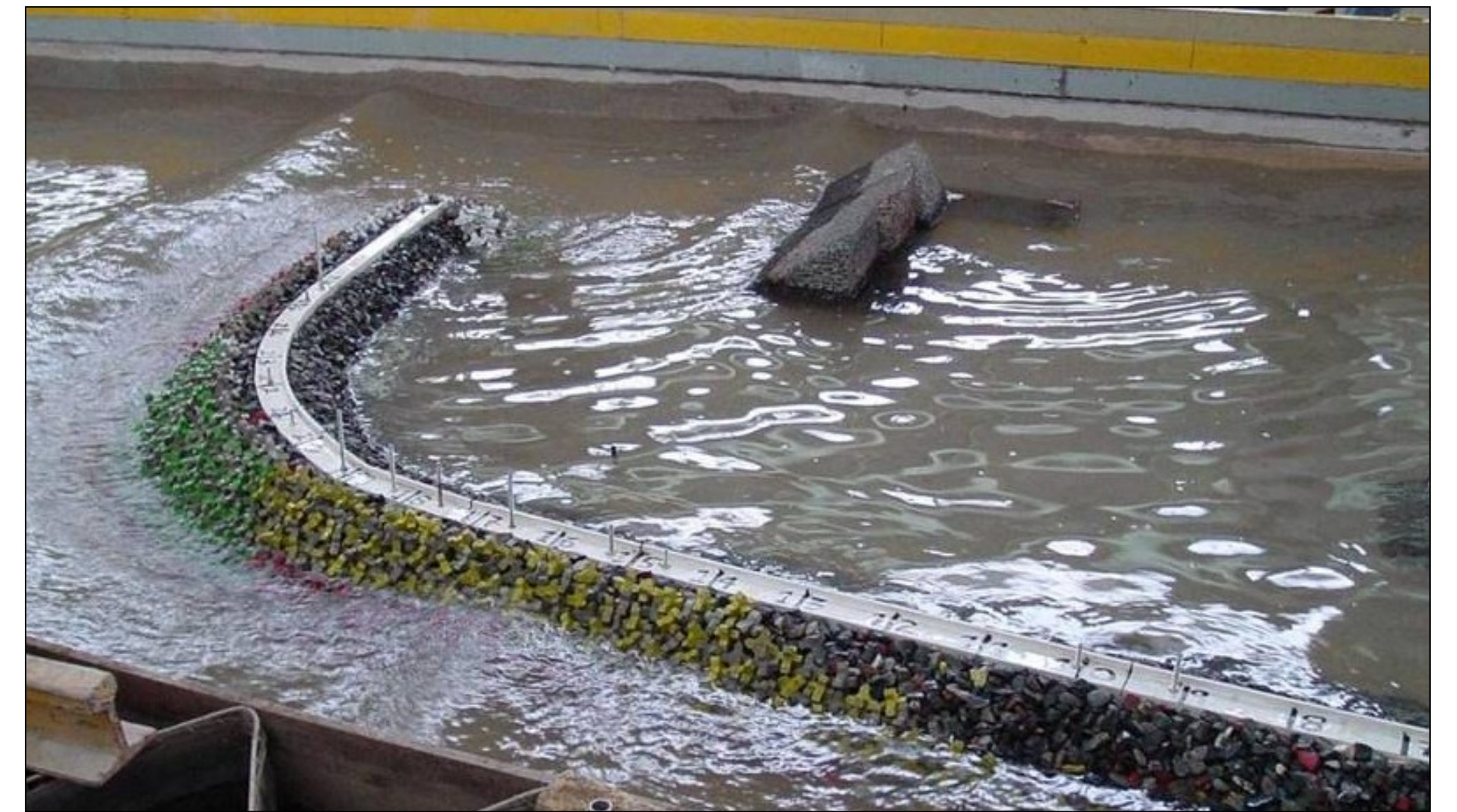
Model tests in a wave basin (Delta Marine Consultants, The Netherlands)
