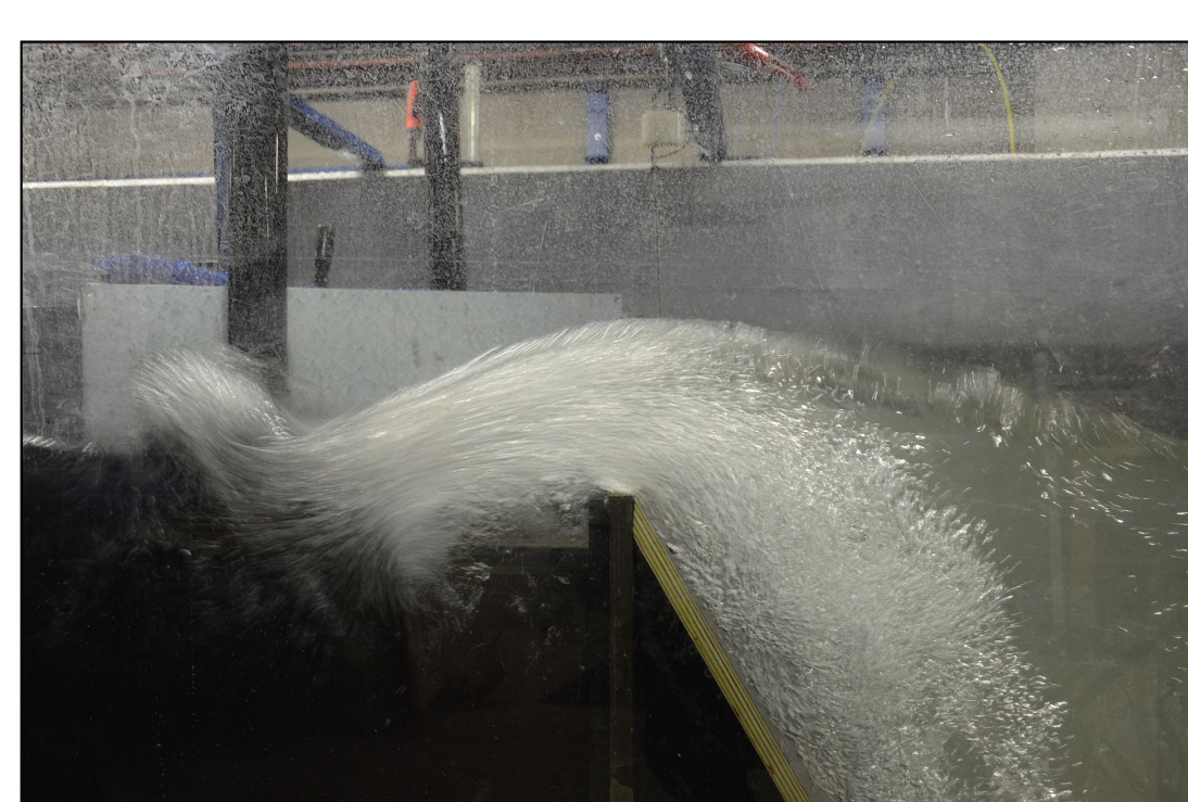
Wave overtopping tests on steep low-crested structures (AWW, UGent)
